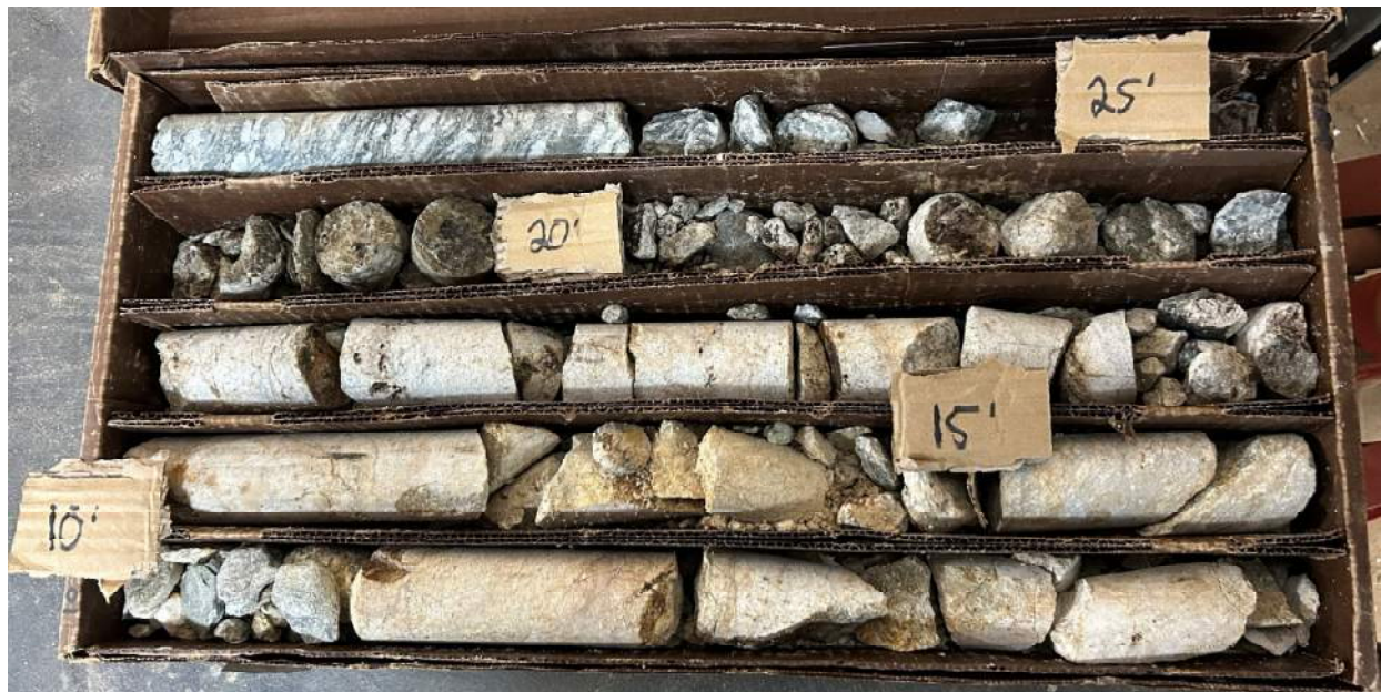
Photograph 1 – Boring B02, 10 feet to 25 feet bgs
